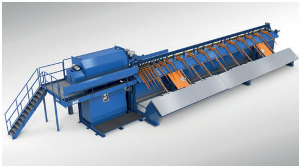
*Pedax processing centre for reinforcing steel fabrication from the coil. The new fully auto-mated system combines a straightening machine with automatic hyperbolic rotors, a double bender and a stirrup bender in one centre.*
