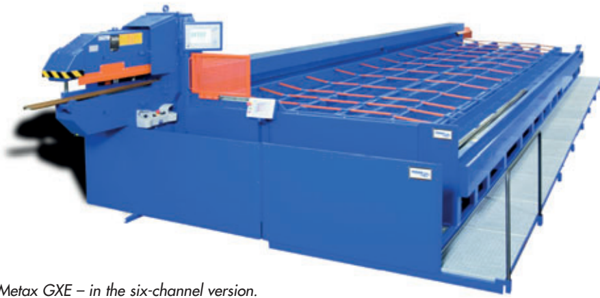
Metax GXE – in the six-channel version. Efficient on account of its great intermediate storage capacity
